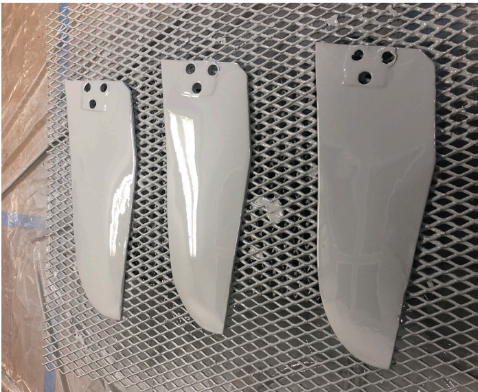
3. Mixing blades coated with Novocoat SC3300 Novolac Epoxy Lining.
